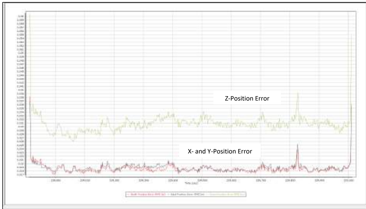
Figure 3.2 Horizontal and vertical accuracy of the Trimble MX7 trajectory.
