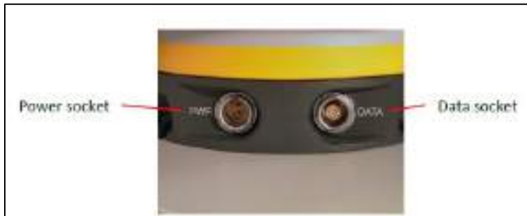
Figure A.6 Photo of Trimble MX7 Sockets for the power and data cables.
