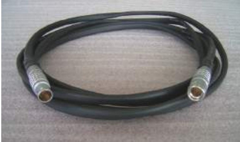
Figure A.5 Photo of the data cable to be connected between the MX7 and power convert unit.
