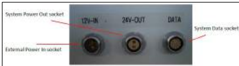
Figure A.7 Photo of 12V-IN power and system data sockets on power converter unit.
